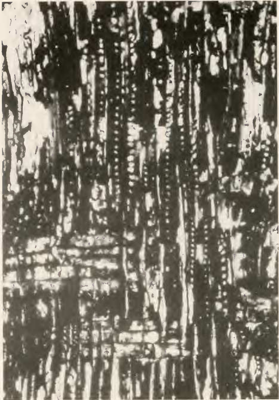
Fig. 19. Radial longitudinal section with bordered pits on radial walls. x 125.
